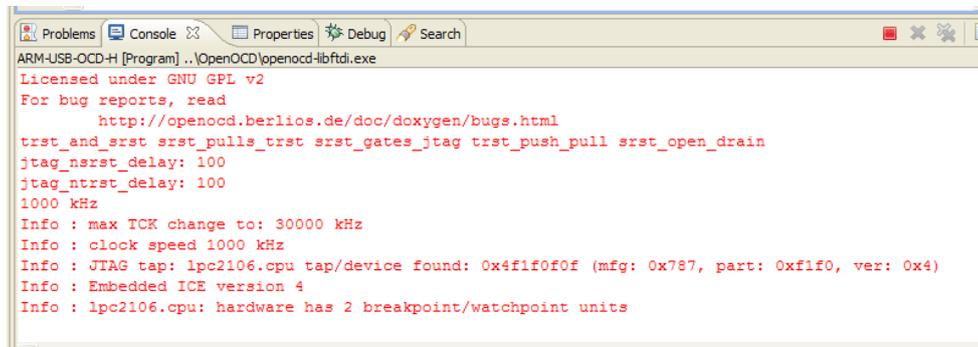
This means that your JTAG is connected to the target and is ready to execute commands.
